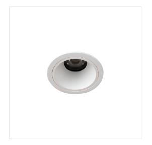
Designed for ultimate precision, the Gusto Rondo delivers a tight beam angle, making it perfect for accent lighting, retail displays, and high-precision tasks. With beam angles of 4° and 6°, a high CRI of 95, and a peak candela of 7500cd at 6°, Gusto ensures exceptional light quality. Its leaf springs provide a secure and stable mounting solution. Choose Gusto for focused illumination where precision truly matters.
